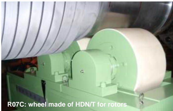
R07C: wheel made of HDN/T for rotors
